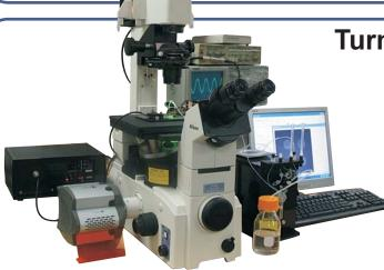
Turnkey Single Molecule Detection TIRF Microscopy System
