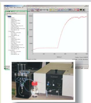
SmartFlow fluidics is recommended for use with TIRF Flow System TA1004, and lightguide-, objective- and prism-based TIRF microscopy flow systems. SmartFlow application window can be conveniently open in one screen with your fluorometer application or microscopy imaging software. SmartFlow facilitates measuring of sensograms and deriving of rate constants k-on and k-off.
